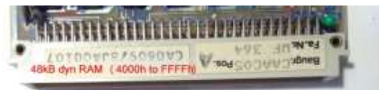
ADAPTER: Addresses access 0000h-BFFFh shift range / hide selection 0000h-3FFFh (off/on) software switching
